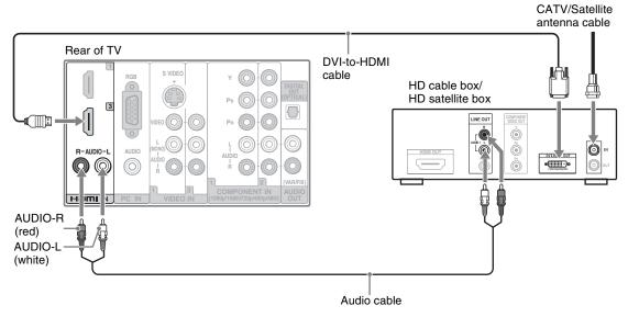
• If the equipment has a DVI jack and not an HDMI jack, connect the DVI jack to the HDMI IN 3 (with DVI-to-HDMI cable or adapter) jack and connect the audio jack to the AUDIO IN (L/R) jacks of HDMI IN 3. For details, see page 15.
